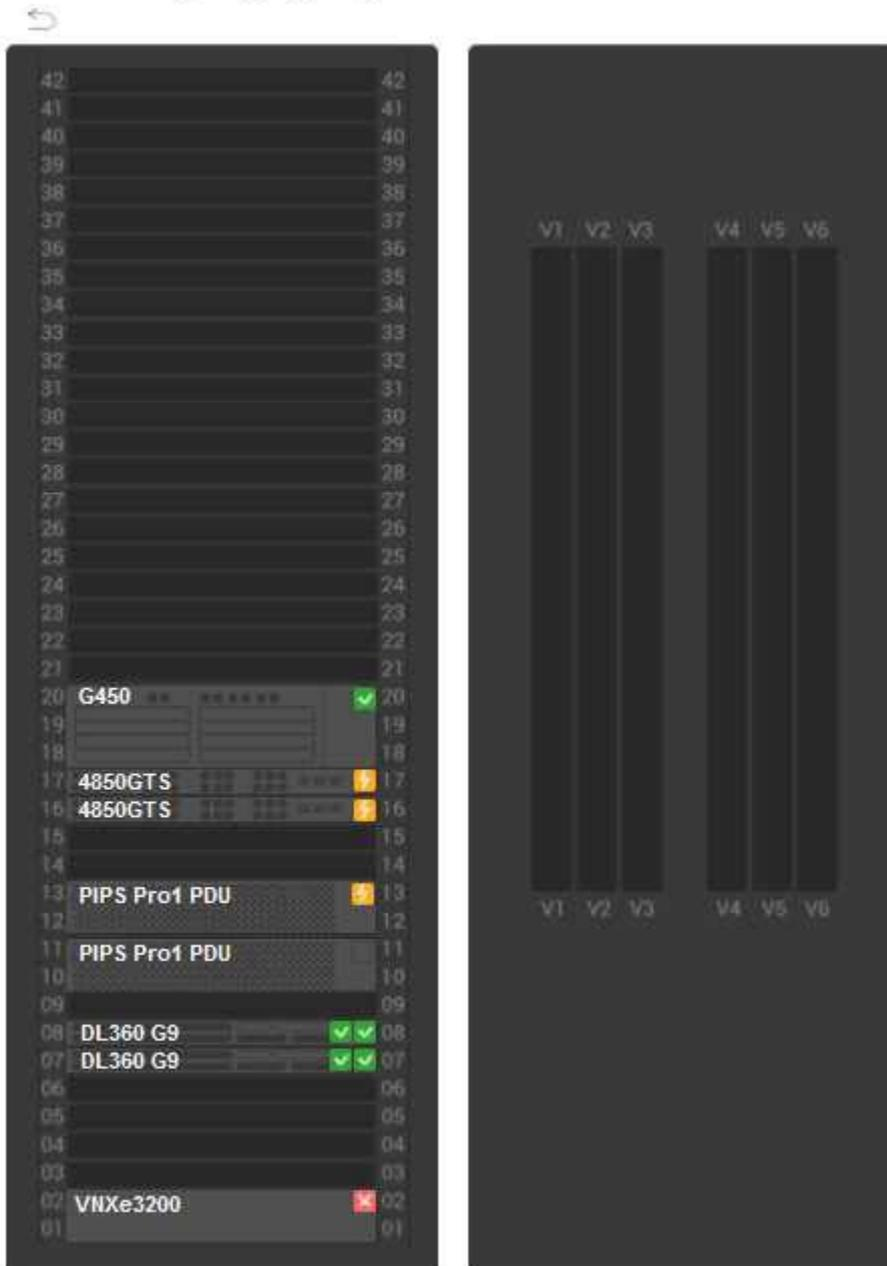
When a support engineer navigates to Orchestrator's Rack View of an ACP 4200 system, the engineer notices that the V1-V6 slots on the right of the diagram are not populated. What could be causing this problem?
